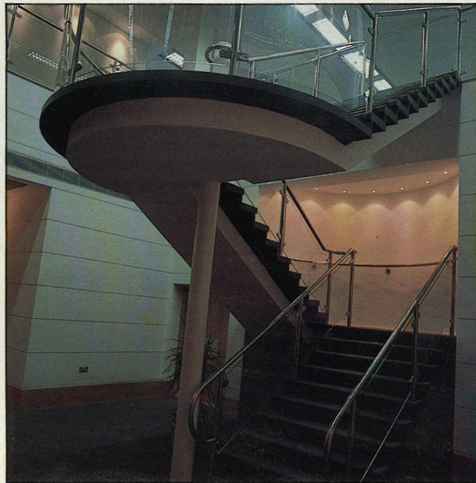
Guildford Business Park: the sculptural staircase revealed in silhouette by use of low voltage fixtures with integral reflectors providing a controlled scalloped effect on the wall.
