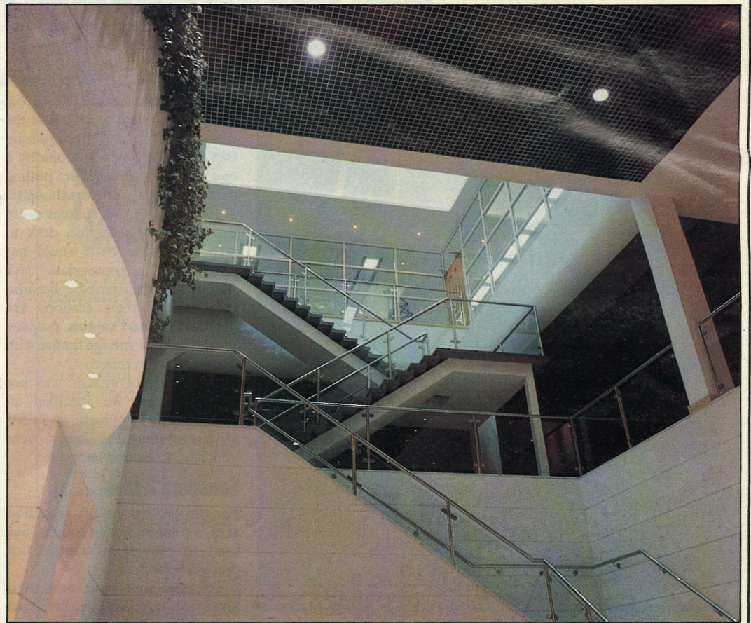
View of Guildford Business Park reception area showing a combination of low voltage sources over the reception desk and on the half landings, with metal halide downlights providing infill lighting.
